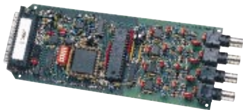
OMB-DBK7 Four-Channel Frequency-Input Card
