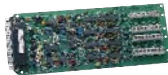
OMB-DBK9 Eight-Channel RTD Measurement Card
